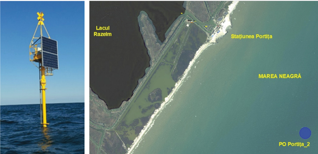
1. Portița_2: Coastal Beacon: the beacon will be mounted at the isobath of (-15.00) m near Portița Resort. The access to Portița_2 will be made exclusively on the water, with the help of the technical maritime ship dedicated especially to the maintenance of all the buoys and coastal beacons that will belong to DANUBIUS-RO.
